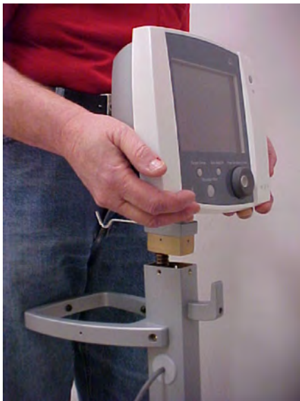
Figure 3.4. Attach the Display Head to the Mast
