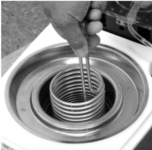
Figure 4.39. Installing the Heat Exchange Coil
