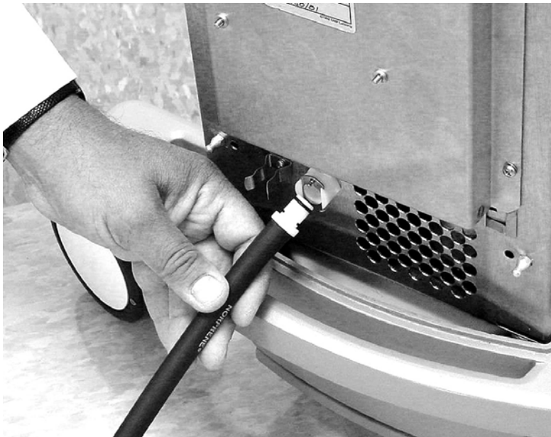
Figure 7.3. Push Hose Into Drain Coupler
