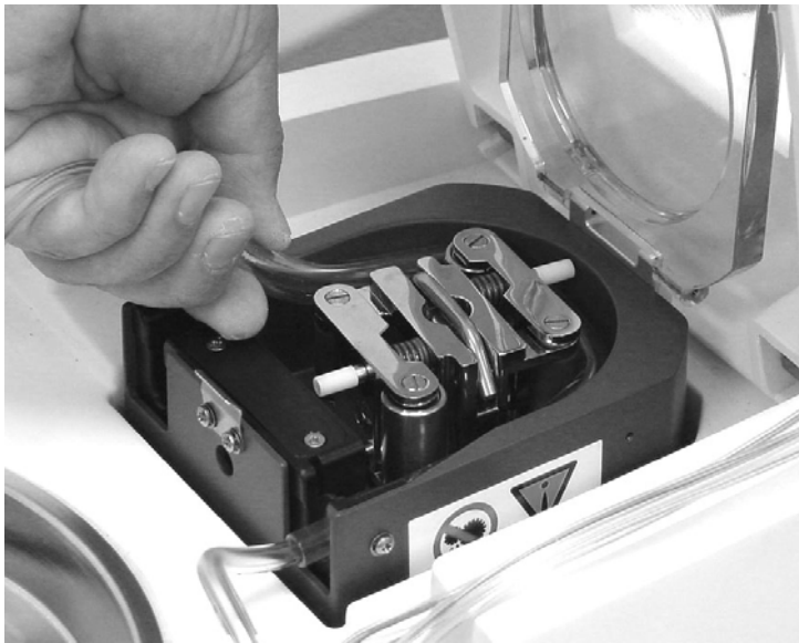
Figure 4.43. Pump Tubing Installation
