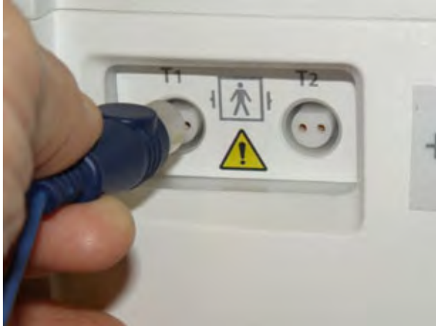
Figure 4.50. Temperature Probe Connections
