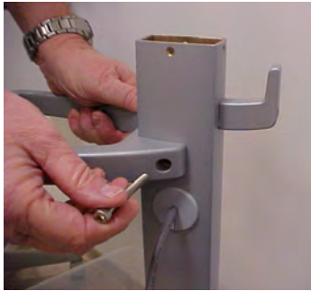
Figure 3.3. Use the Long Bolt and Center Screw to Attach the Handle
