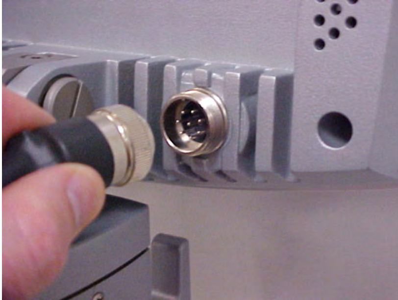
Figure 3.5. Plug the Control Cable Into the Socket
